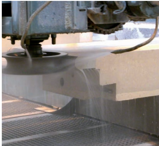
Treatment of the flight of stairs with a diamond drilling mill
