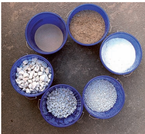
Concrete aggregates: (1) white cement, (2) marble 2/8, (3) marble 8/16, (4) marble 16/35, (5) quartz sand 0/1, (6) sand 0/2
